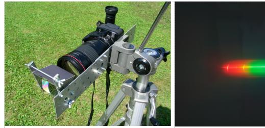
To record the spectrum over the long side of the image and parallel to the vertex angle of the contact point (352 °), the camera system was tilted by 90 °.
